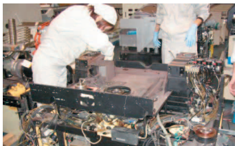
Disassembly process for end-of-life equipment
