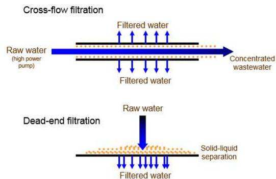
Fig. 2 Cross-flow filtration and dead-end
