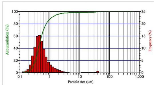
Fig. 1 Particle sizes of silicon fragments contained in the wastewater from the dicer.
